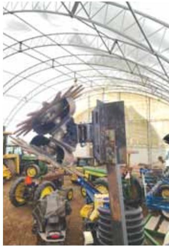
Kroll put row cleaners onto his planter marker arm to mark his no-till fields to stop furrowing.
