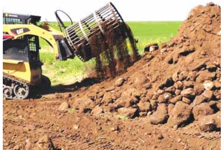
Quicker Picker rock picker barrel rotates as dirt and debris fall through holding the rocks inside.
