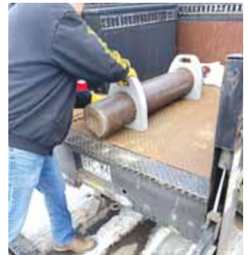
Foam handles slide over tank to allow for carrying and transporting welding tanks.
