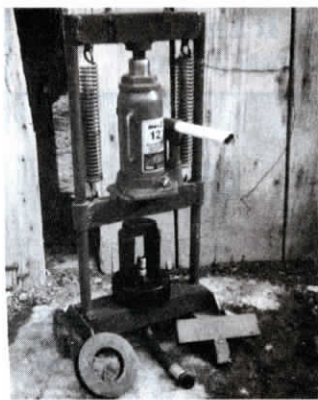
Vesco's home-built shop tool can be used to repair hydraulic hose (left), baler belts (right), or it can be used as a press on bearings or U-joints.
