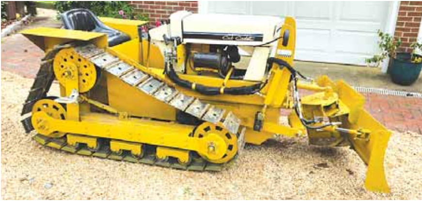
Smith used the frames and rear ends from two Cubs to make his dozer frame about 2 ft. longer than the original with a drive axle and differential at both ends.
