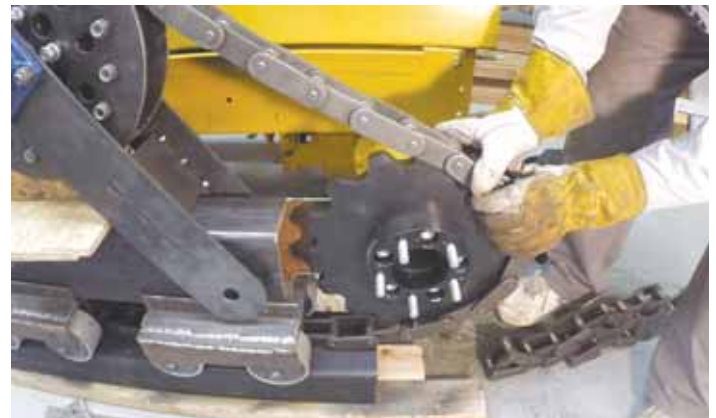
To make the track, Smith bought heavy duty 2 1/2-in. chain and cut out steel pads on a CNC table to weld to the chain.
