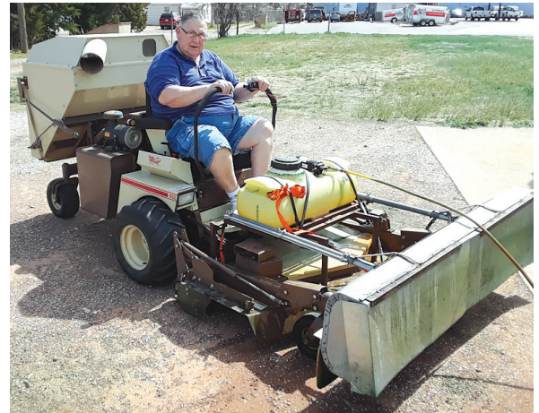
Spray can be delivered via a 10-ft. hose with a wand or the spray hood. A quick connect lets Penick detach the hose and direct the flow to the spray hood.
