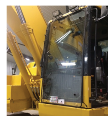
Tractor Guard window protection systems are designed to protect your tractor’s windows from flying debris.
