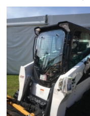
Tractor Guard window protection systems are designed to protect your tractor’s windows from flying debris.
