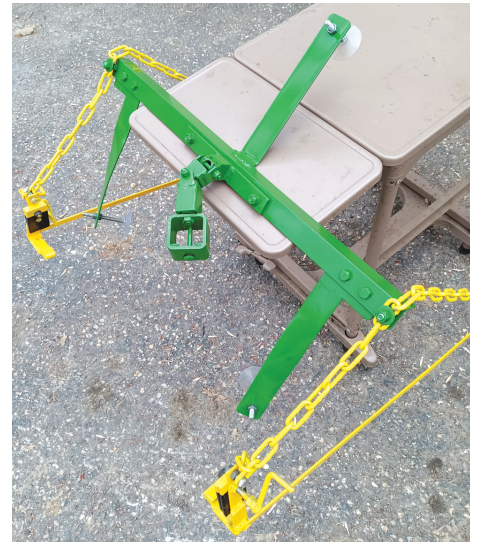
Bunniss hood remover is articulated in four directions, swivels, and will stay where he sets it, making it possible to place the hood back on the tractor, level on all planes. It’s fully adjustable and can be used for large and small tractors.
