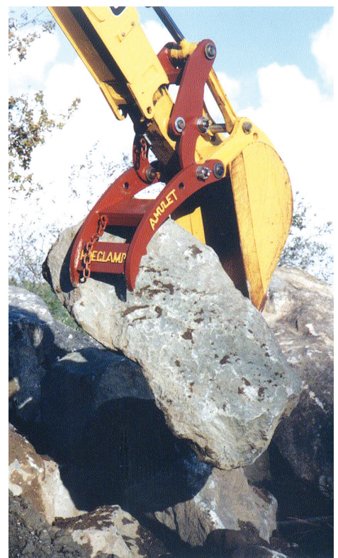
HoeClamp moves as bucket moves. Lund says it’s easier to use than a “hydraulic thumb.”
