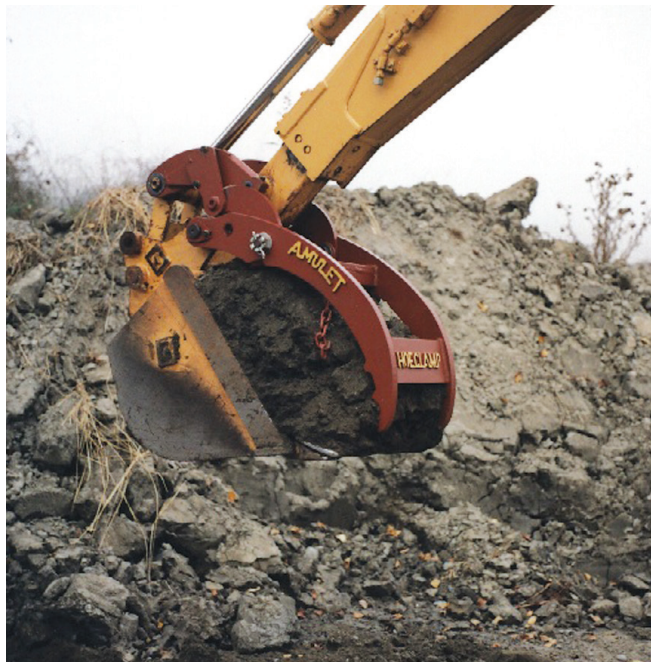
HoeClamp moves as bucket moves. Lund says it’s easier to use than a “hydraulic thumb.”
