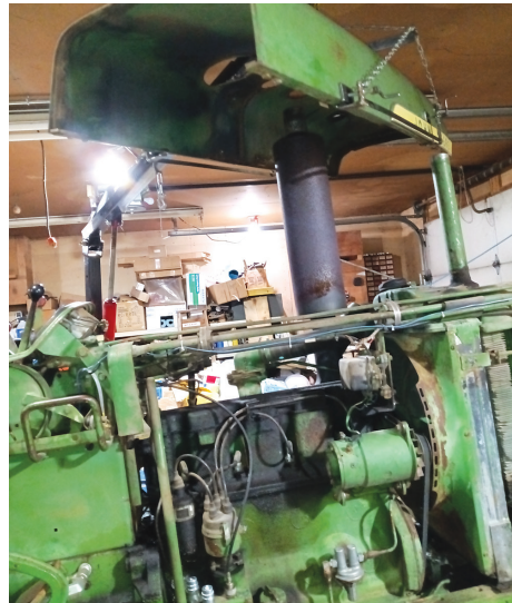
Bunniss hood remover is articulated in four directions, swivels, and will stay where he sets it, making it possible to place the hood back on the tractor, level on all planes. It’s fully adjustable and can be used for large and small tractors.
