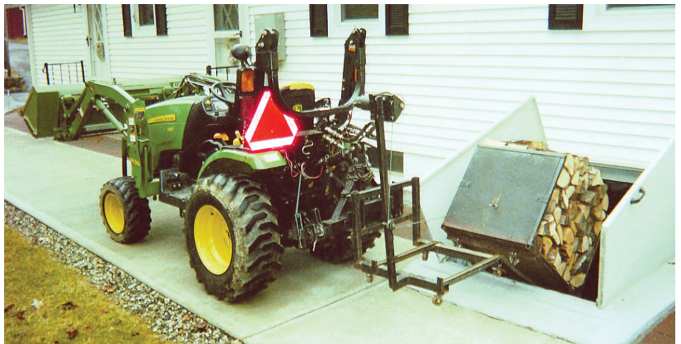
Metal firewood box rides on caster wheels that rides on steel tubing track down stairs using a winch.
