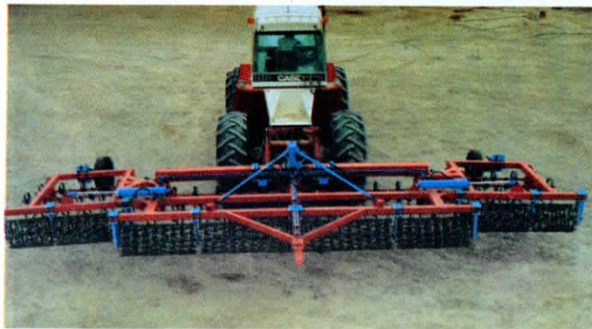
The 28-ft. wide harrow has a 17-ft. main frame with 5 1/2-ft. wings.
