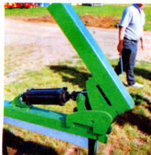
Hinge kit lets you use common 8-in. cylinders to fold up tillage equipment and is designed with cam-type lift levers.
