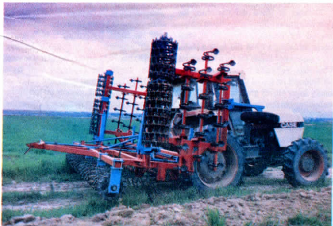
Harrow has three rows of S-tines fitted with 7-in. sweeps followed by one row of "crowfoot" rollers.
