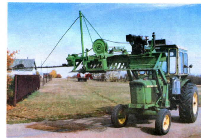
Mower is belt-driven by Briggs & Stratton gas engine that mounts on loader.
