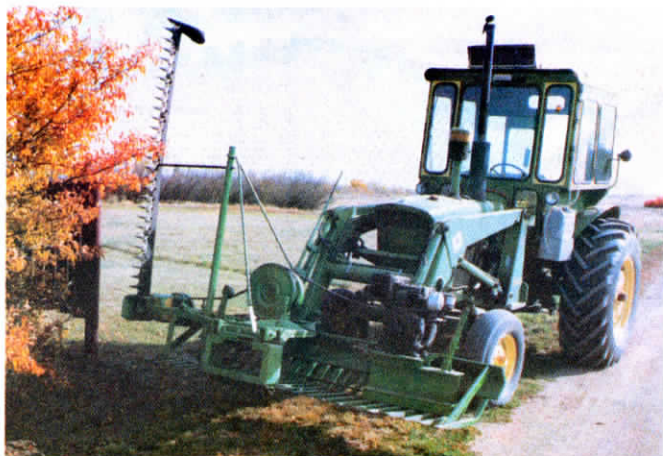
The "Bush Wacker" can trim a mile of hedge in about 6 hours, trimming both sides and making two passes over the top.
