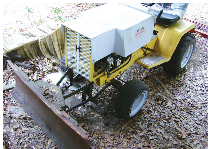
Rawls used a Harbor Freight 6-hp. engine and IH 404 clutch to rebuild his Cub Cadet.
