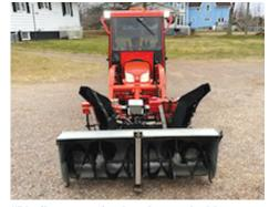
"I built a mounting bracket on the blowers to match the one on my tractor," McCallum says. "I just take off my quick attach bucket, drive up to the blowers, put in two pins, and plug in the power cord from the tractor."
