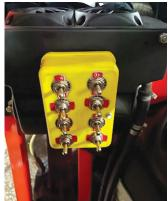
To power the units, he mounted a control box in the cab containing 18 wires plus the positive and negative from the tractor.
