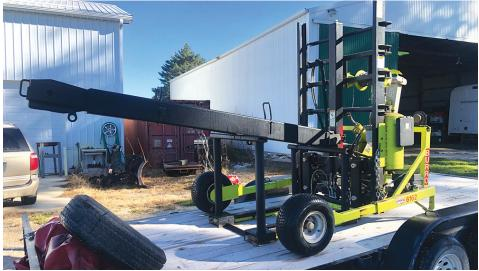
To support his extended boom, Boyce welded a framework of 1/2-in. thick by 3-in. boiler pipe for upright legs and upper horizontal supports. He added metal pockets for the forklift tines to slide into to lift the unit.
