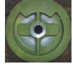
Allen Machine Works casts new flywheels for 720 and 730 diesels. They rebuild other models using their Taper-Loc Hub.
