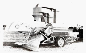
New combine's 4 ft. wide vacuum pickup features a full width adjustable roller to keep vacuum at a constant distance from the ground.
