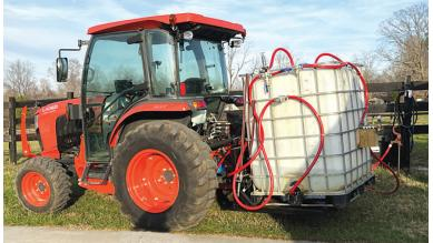
300-gal. tote was the starting point. From there, Davis went to Amazon and picked out what he needed, such as an 8-roller, ptodriven pump with 100 gpm flow.
