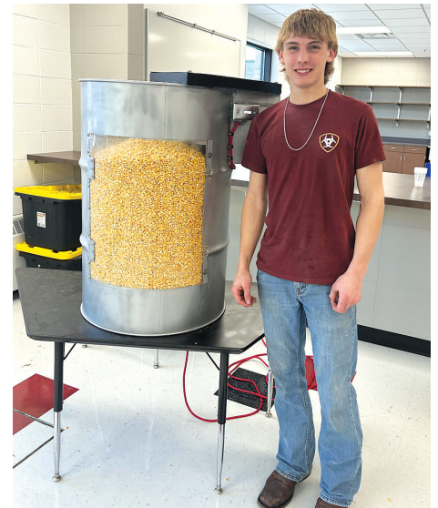
Mason Gahler developed his Grain Gyre to move grain in the bin making it less likely for grain entrapment.
