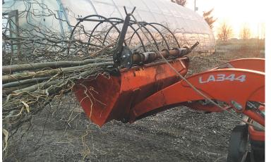
Currently, the tines fall 8 to 10 in. ahead of the bucket edge. **Tschetter plans** to add removable teeth to extend the bucket's reach.
