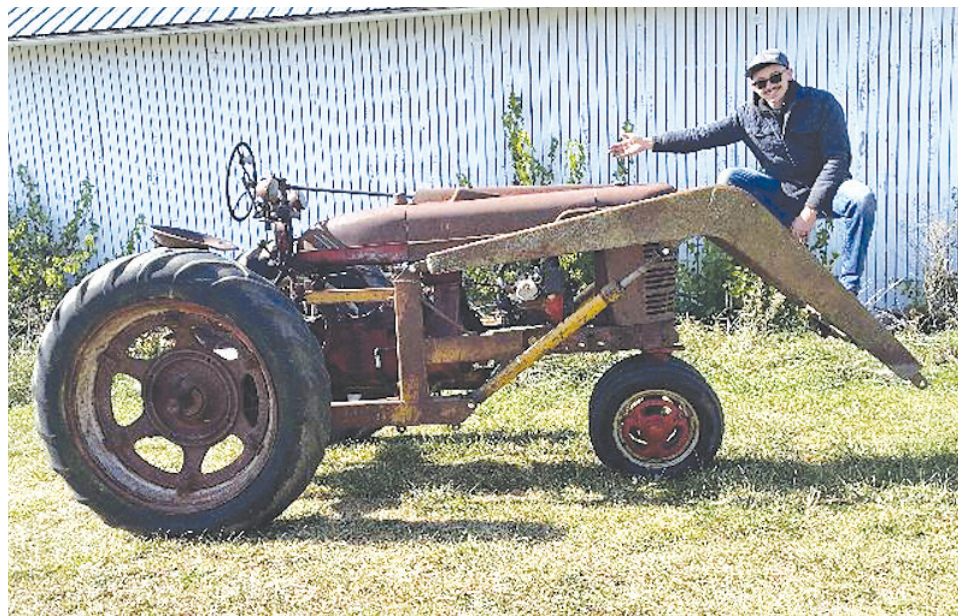
Lindemer’s 1948 Farmall M uses an 11-hp. Honda engine and transmission from an old Crosley car.
