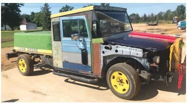
Imhoff used a pickup and parts from a semi, combine and tractor to create his rat rod.
