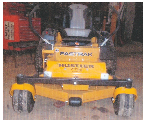
Lacey modified the front suspension of his mower for a more stable ride.
