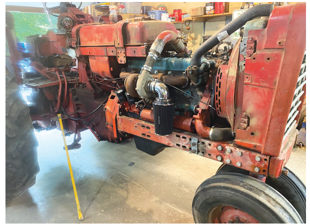
756 Farmall repowered with DT360 engine from an International school bus.
