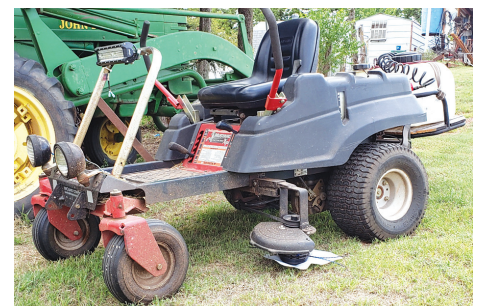
Krueger made an extension from 3-in. box tubing to mount the power head from an old DR trimmer head to the side of the zero-turn.
