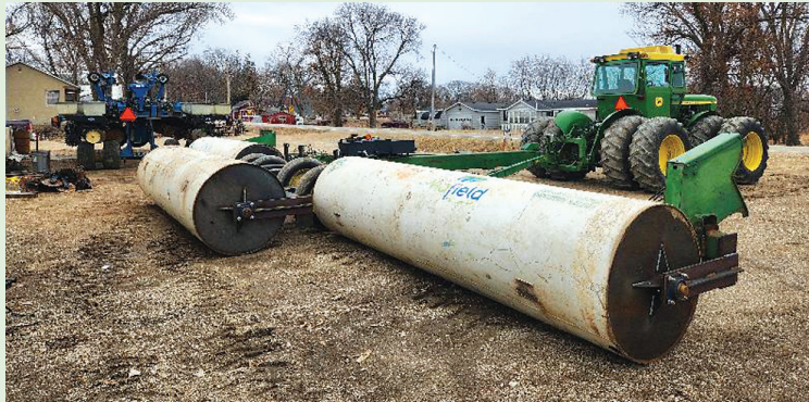
Farmer built a three-section 42-ft. wide field roller using the frame and wheels from a Deere 7000 16-row planter and three used anhydrous tanks.
