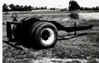
Dolly is available with long or short tongue, and with new or reconditioned 20,000 lb. axle.
