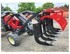
by 8-in. hydraulic cylinder with a large jaw opening of 36 in. The floor of the grapple is approximately the same length as the bucket floor of the tractor. Because it doesn't curve up at the end, users can get under the material they wish to pick up.
