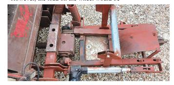
"I incorporated a 1-in. keyed shaft for the mower pot. The gearbox mounts to the pto shaft with a keyed coupler."
