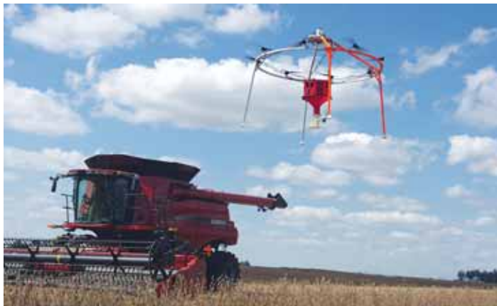
Leitgen's custom build drone can carry a 30 lb. payload and has a 65-in. dia. aluminum hoop frame.
