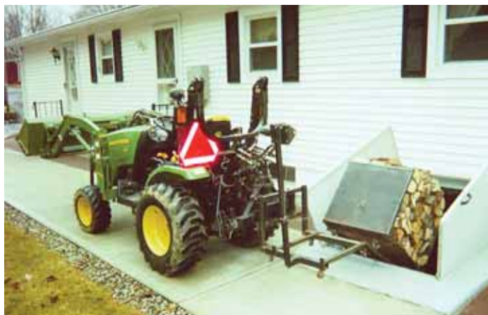
Metal firewood box rides on caster wheels that rides on steel tubing track down stairs using a winch.
