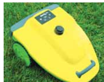
Lawn care robot can carry 1.2 liters of herbicide and cover up to 1 acre.
