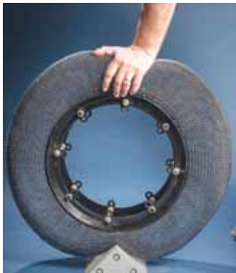
Tires made from Nitinol were developed by NASA and can flex as needed while handling heavy loads.
