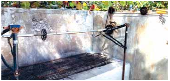
Cronk used old bicycle chains, sprockets, and other parts to make this spit for roasting a 50-lb. hog.
