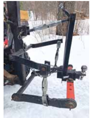
"I designed the 3-pt. so I can unplug the electrical connection, pull the pin on the receiver hitch and move the 3-pt. to any other 2-in. receiver hitch," says Sieting.
