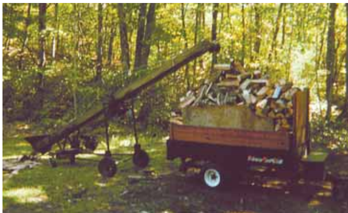
16 ft. conveyor can move firewood about 10 ft. high to drop into trailers or trucks.
