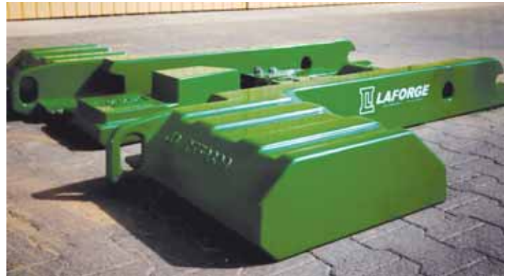
LaForge makes a drive-over ballast that lifts securely to the undercarriage of Deere 7R tractors.
