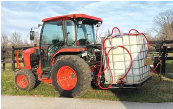
300-gal. tote was the starting point. From there, Davis went to Amazon and picked out what he needed, such as an 8-roller, pto-driven pump with 100 gpm flow.
