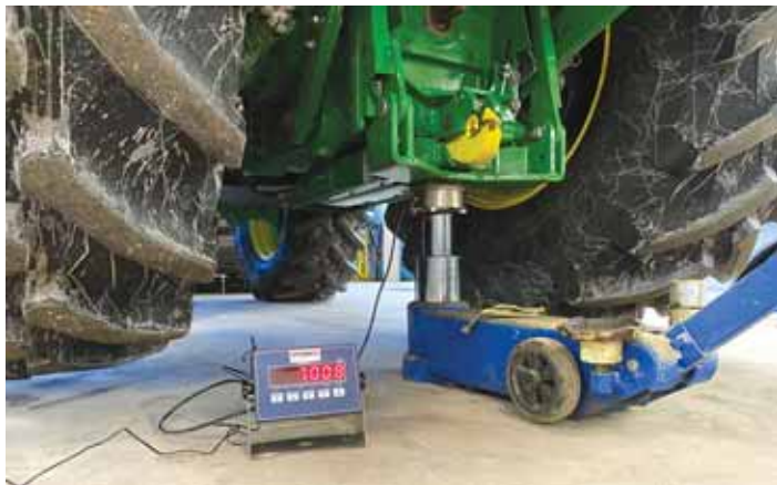
The Newton includes a compressed air-driven jack with a mechanical interface between it and a strain gauge (wave or load cell).
