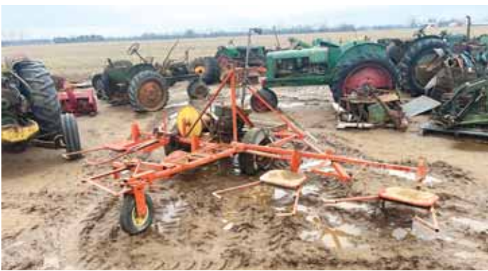
Main frame is 11 ft. long and 13 1/2 ft. wide. It’s powered by a 7-hp. Briggs and Stratton engine. A large pulley on the engine drives a small pulley on the Wheel Horse transmission.
