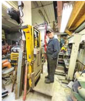
Shop lift made from an old forklift with a lift capacity of around 2,000 lbs.
