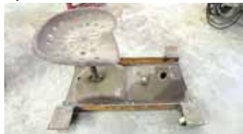
Shop dolly made from the seat and gearcase of a Farmall F20.
