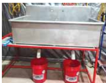
Stainless steel sink on a metal stand used to clean rusty tractor parts.
