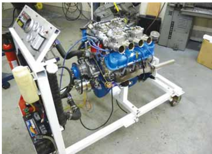
Frame uses adjustable crossbars with upright arms with motor mounts for the engine to be tested. At the front of the stand, two upright arms with a crossbar provide support for a control panel.
