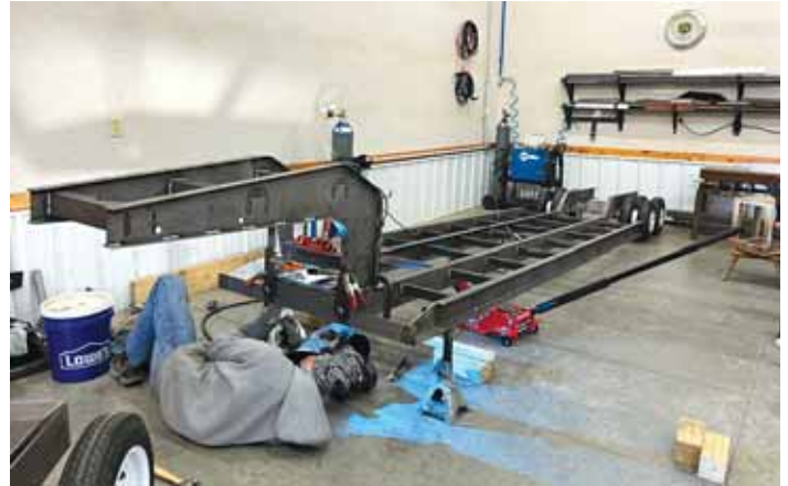
Mini trailer frame beams use 2-in. strap steel welded to vertical 1/4-in. plate steel.
