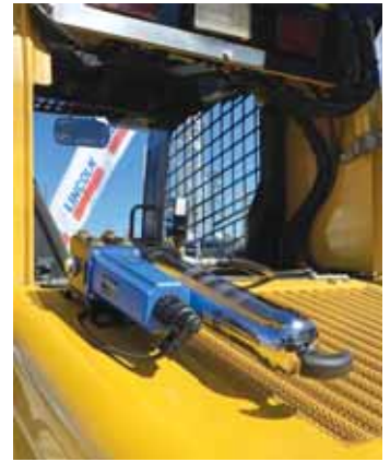
A cab-mounted controller alerts the operator when a tube change is required.
