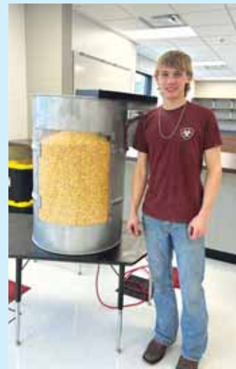
Mason Gahler developed his Grain Gyre to move grain in the bin making it less likely for grain entrapment.
