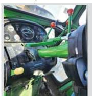
Brad Farmer made a custom bracket for the steering column of his Deere 8440 so he could install a guidance system on the tractor.
