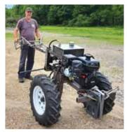
Tractor has zero-turn capability with controls at the hand grips.
