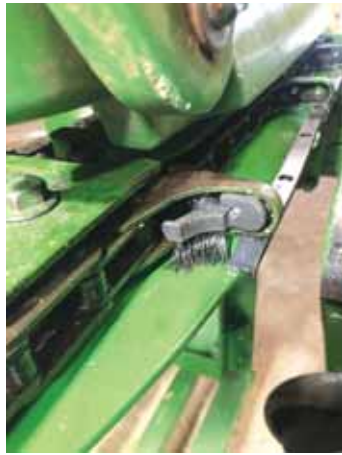
Black poly rail and brush on a gathering chain are part of the kit.
