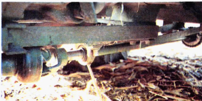
The pto shaft is knuckled twice under the tractor.
