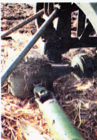
The chopper gearbox is turned around to attach to the pto.
