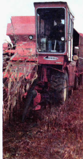
Corn stalks are cut off about 9 in. off the ground and the whole plant goes through the combine.
