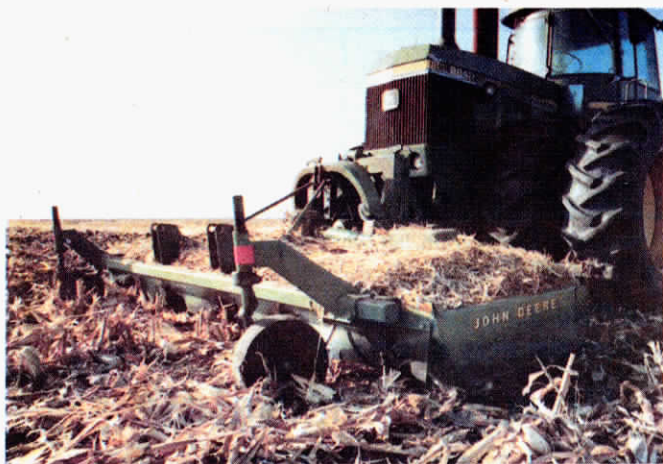
The chopper's rear wheels were moved to the front of the machine.
