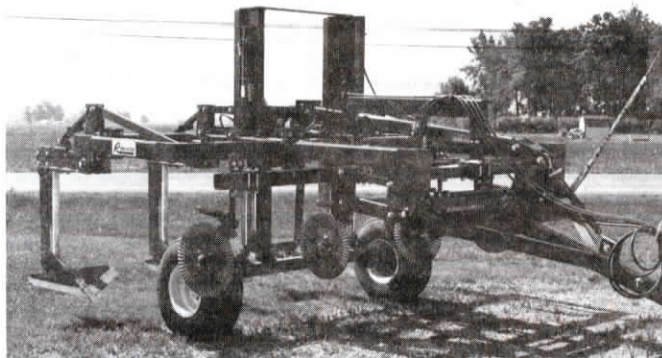
Unit's 30-in. wide blades are spaced 12 in. apart to shatter soil compaction zone.
