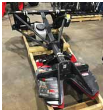
Tree shear can handle up to a 9-in. dia. tree.
