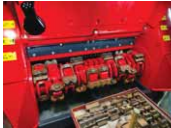
Stones are pounded against hydraulically adjustable anvils using up to 14 hammers.
