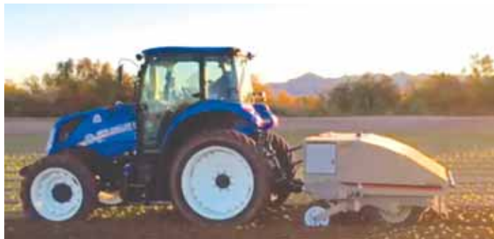
Stout "Smart Cultivator", pulled by a 100-hp. tractor, identifies weeds by cameras using Artificial Intelligence software, then plucks them out from around productive vegetables.
