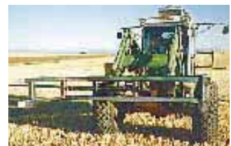
Bale clamp carries two big square bales at a time. It has one telescopic arm that’s extended out sideways by a 3 by 24-in. hydraulic cylinder.
