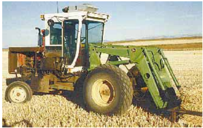
Self-propelled “clamp loader” was built from a Massey Ferguson 510 combine and is equipped with a Deere 260 loader and the cab off a 1980 Gleaner L combine.
