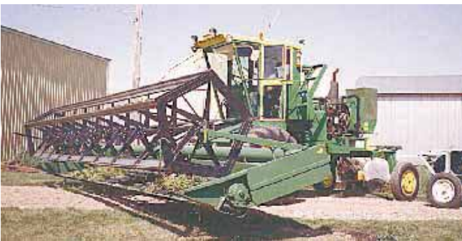
Darker rebuilt an older-model Versatile 5000 hydrostatic drive combine, mounting a 30-ft. McDon double swather table on front that’s driven by hydraulic motors.
