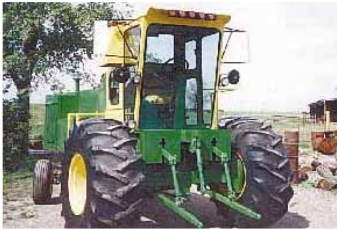
Kirby converted a Deere 55 combine into a tractor with 3-pt. hitch and pto on front.
