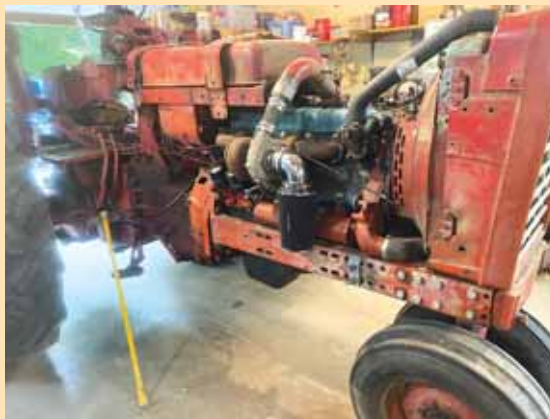
756 Farmall repowered with DT360 engine from an International school bus.
