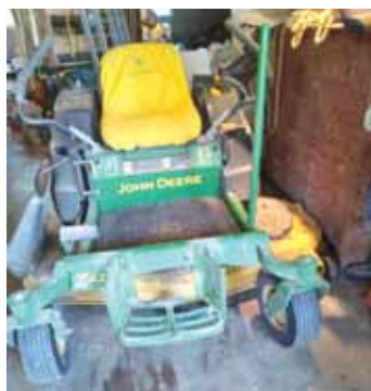
Ehemann put a step on the front of his zero-turn mower to make it easier to get on and off.
