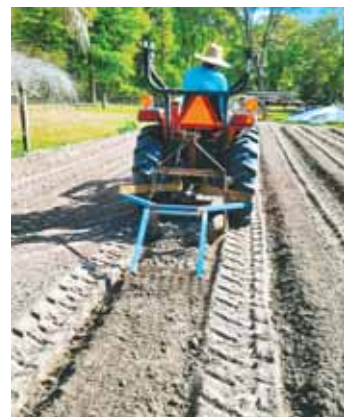
Lynn fabricated an attachment out of a scrap piece of heavy-duty expanded metal that flattens the garden bed and leaves a smooth top for planting.
