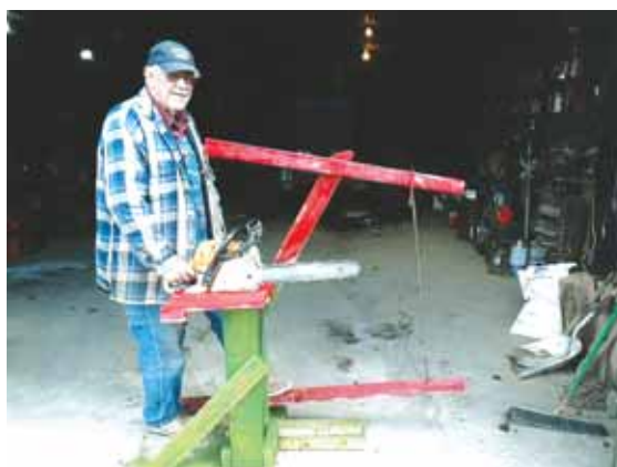
Starter uses a series of levers to pull on a cord connected from a foot pedal to the chainsaw's starter.
