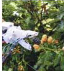
Medical robotic techniques were used to develop this 3-fingered berry picker.
