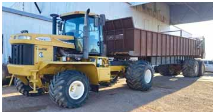
Trailer's gooseneck-style hitch mounts to a receiver on a 4-WD 8144 Terra Gator. It originally carried a large bulk tank and applied dry fertilizer.
