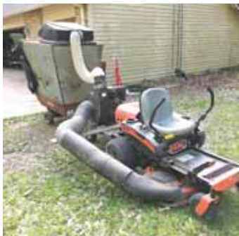
Day used a Bluebird vacuum and Snapper Bag-N-Wagon to make his mower vac.
