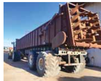
Spreader can haul 40 to 45 tons per load, reducing the number of trips required.
