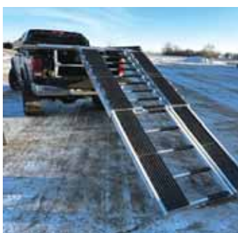
10-ft. telescopic ramp makes it easy to load equipment.
