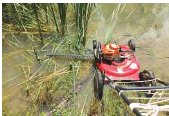
Day's tool cuts down weeds and leaves the stalks long enough for easy removal.
