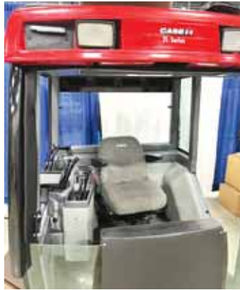
Upholstery kits are made to fit various tractor and combine models with little to no modification.
