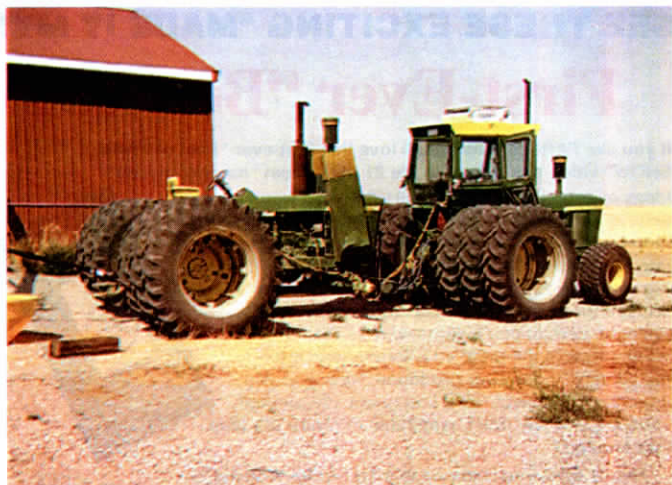
Doubled-up Deere 5020's provide low-cost power for pulling air seeder, seed hopper.
