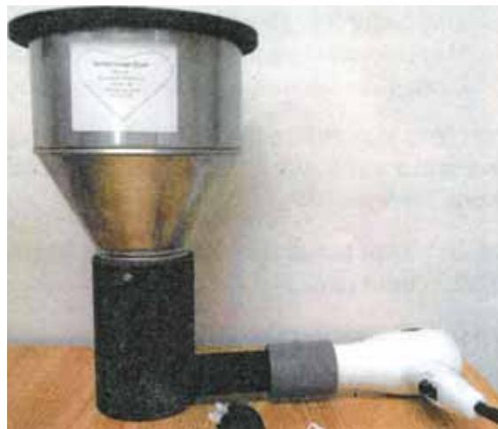
You weigh the dryer and approximately 200 grams of forage, corn, silage or haylage. Then connect and run the dryer for 15 minutes to 1.5 hours depending on the sample.
