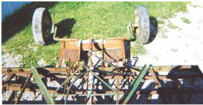
Carrier is designed using a hydraulic cylinder to support and lift either a drag or dirt blade.
